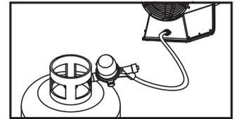
The supply pressure is provided by the pressure regulator supplied as a standard item, and corresponding to the technical specifications table.
