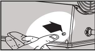
4. After igniting the flame, keep the gas button pressed for 15 seconds to activate thermal safety devices.
