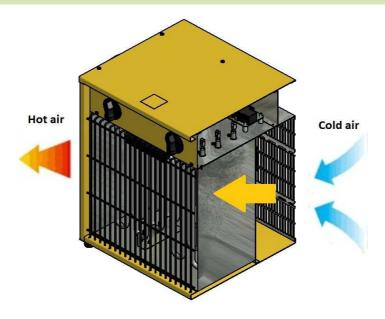
The device works on the principle offorced convection . The air flow is forced fan. Cold air is drawn in the back of the unit. Further washes flowing from the heater receives heat. The heated air is expelled in front of the heater. The device has a thermostat for the regulation temperatures 5-35  $^{\circ}$ C. The unit area equipped with thermal protection with reset. The unit features: ventilation, heating with half the power, heating at full power. Device has cooling thermostat.
